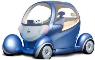
This concept car was initially shown in 2005. It has a 360 degree rotating three-seater cabin and eliminates the need for reversing and so makes parking a breeze. Powered by a lithium-ion battery makes it economical to run. The design includes a large door for easy access and huge windscreens and windows for increased visibility.
